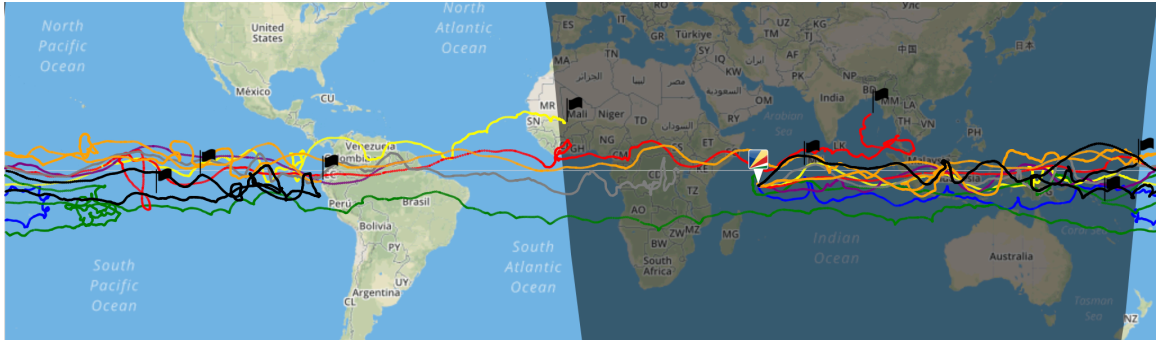
Figure 3 Flight trajectories of the eight Strateole-2 balloons during the technology validation campaign 12 November 2019 through 28 February 2020. The 06_STR1 balloon carrying the ROC2 receiver is shown in yellow.
