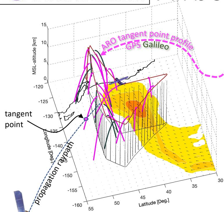
ARO retrieves a profile of refractivity values at the midpoints of the raypaths each time a GNSS satellite sets.
