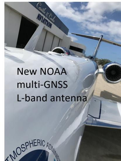
NOAA Grav-D real-time GNSS/IMU positioning system
