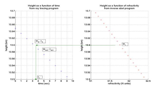
linear interpolation:  $t_i = t_k + \frac{(t_{k+1} - t_k)}{(ht_{k+1} - ht_k)} \cdot (ht_i - ht_k)$
